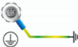
Figure 2: Socket-outlet protective earthing connection
