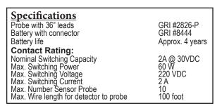
2826FS Normally Open or Normally **Closed Contacts to External Device** Sensor **Sensor Probes** Sensor Normally Closed **Relay Contacts** Common Normally Open 3 V Battery GRI#8444 **Sensor Probe** 0 **Sensor Probe**
