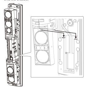
2 Turn the optical unit 90 degrees and tighten the screws (both sides).
