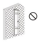
Do not allow the infrared beam from another detector to reach the receiver.
