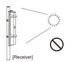
Install the unit at least 1 m (3.3 ft.) away from the wall or fence that may be running parallel to the beam.
