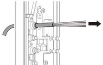
(4) Cut the excess portion of the banding band.
