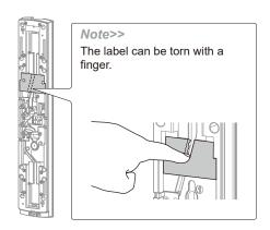
Route the cable alng the wiring groove and draw the cable through the cutbush.
