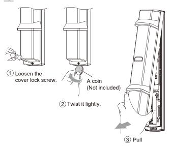
Remove the main unit from the chassis.
