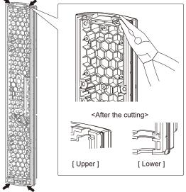
Pull the waterproof packing (x2) marked as "①" at the center of the chassis.
