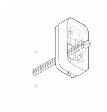
7. If installing chime wires, insert the chime wires into terminals and use a screwdriver to secure them.
