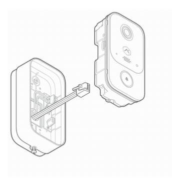
9. Gently insert the main assembly into the wall mount assembly, ensuring that wires are not pinched and there is no excess cable in the doorbell. Firmly press the main assembly until it is completely seated.
