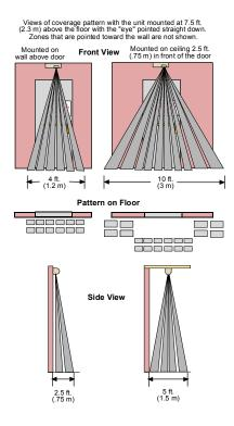
The higher the unit is mounted, the larger the coverage area. Do not mount the DS160 more than 15 ft. (4.6 m) above the floor.
