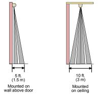
If the DS160 is mounted on the wall above the door, you can move the coverage pattern away from the wall by rotating the detector's lens.
