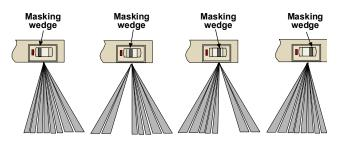
To insert a masking wedge, insert the bottom peg first. Then press on the center of the wedge until it snaps into place.
