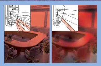
By utilising Optex Advanced Optical Technology, the DX-40/60 create evenly distributed sensitivity throughout the detection area.
