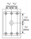
Mark Holes for Drilling Using the back, mark mounting and wiring holes.
