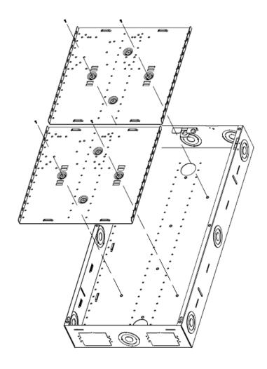
KT-MP500 Case: 3.Installing two plates in a previous cabinet version without lateral holes:
