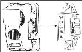
The access holes are provided in the back of the terminal block to allow the voltage to be measured directly without removing the device. Typically this would be done at the end of the line to confirm design criteria. Most measurements will be taken using the S+ and S- locations although access is provided to other locations. **NOTE: Care should be taken to not short the test probes.**
