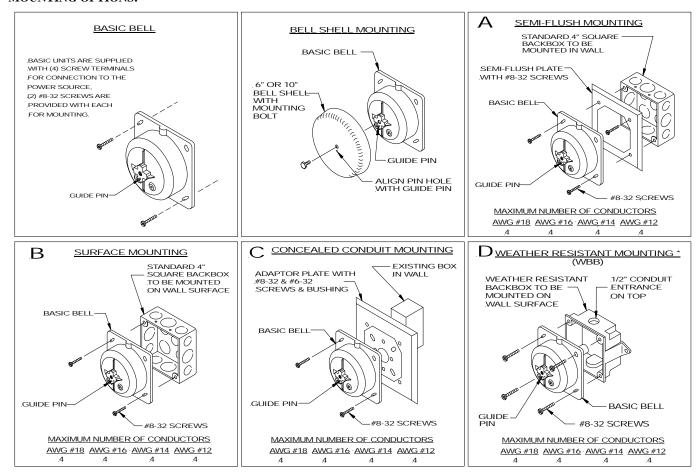
\* Suitable for outdoor use with the WBB Weatherproof backbox (see Mounting Option D).
